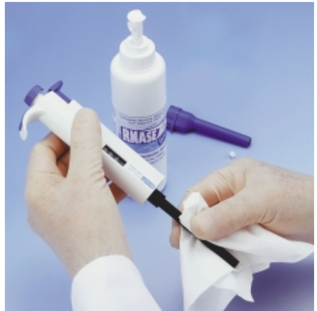
Fig. 5. RNase contamination can be removed by specific RNase zap solution safely, easily and quickly.
