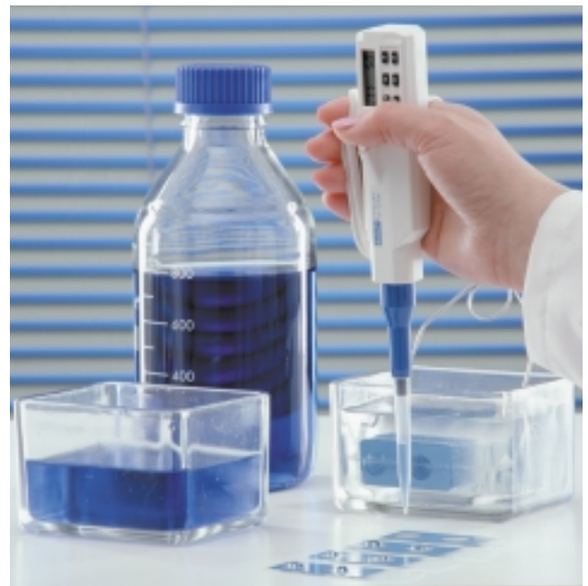
Fig. 1. The benefits of an electronic pipettor are in its ergonomics.
